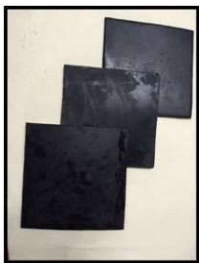
Non-Newtonian sheets developed for Impact Resistance in Cricket
