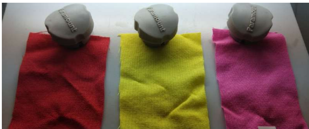
Wool Fabric dyed with Synthesised Fluorescent Dyes (Under 366nm)
